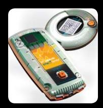
The Primer's STM32 drives ergonomic, MEMS-based controls (navigate by tilting the tool left, right, backward or forward) for fun, easy control of demonstration firmware including graphical user interface and games. The task scheduler firmware and demos provide implementation of low-level functions driving a range of STM32 peripherals, plus features for dynamic loading and management of new applications. All demos (C sources and project) and more future demos are available at www.stm32circle.com.
