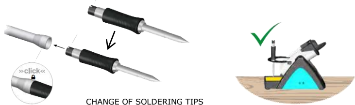
CHANGE OF SOLDERING TIPS IN A COUPLE OF SECONDS (WITHOUT TOOLS)
