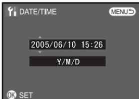
**2** Move to the item you want to adjust by using ◀ / ▶ on the four-way button, and adjust the value of the item by using ▲ / ▼ on the four-way button.
