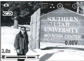
**2** Keep pressing the shutter release button halfway down and recompose your picture.
